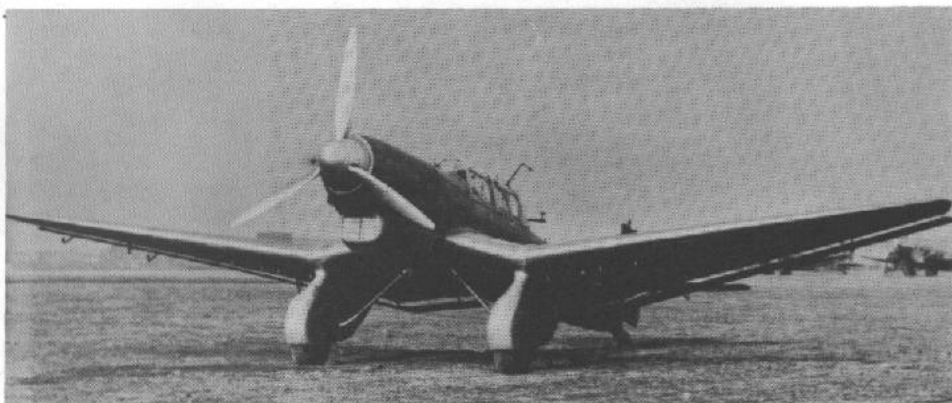
Design prototype of the Stuka series, the Ju 87 V-1 employed a British Rolls Royce Kestrel V engine.
