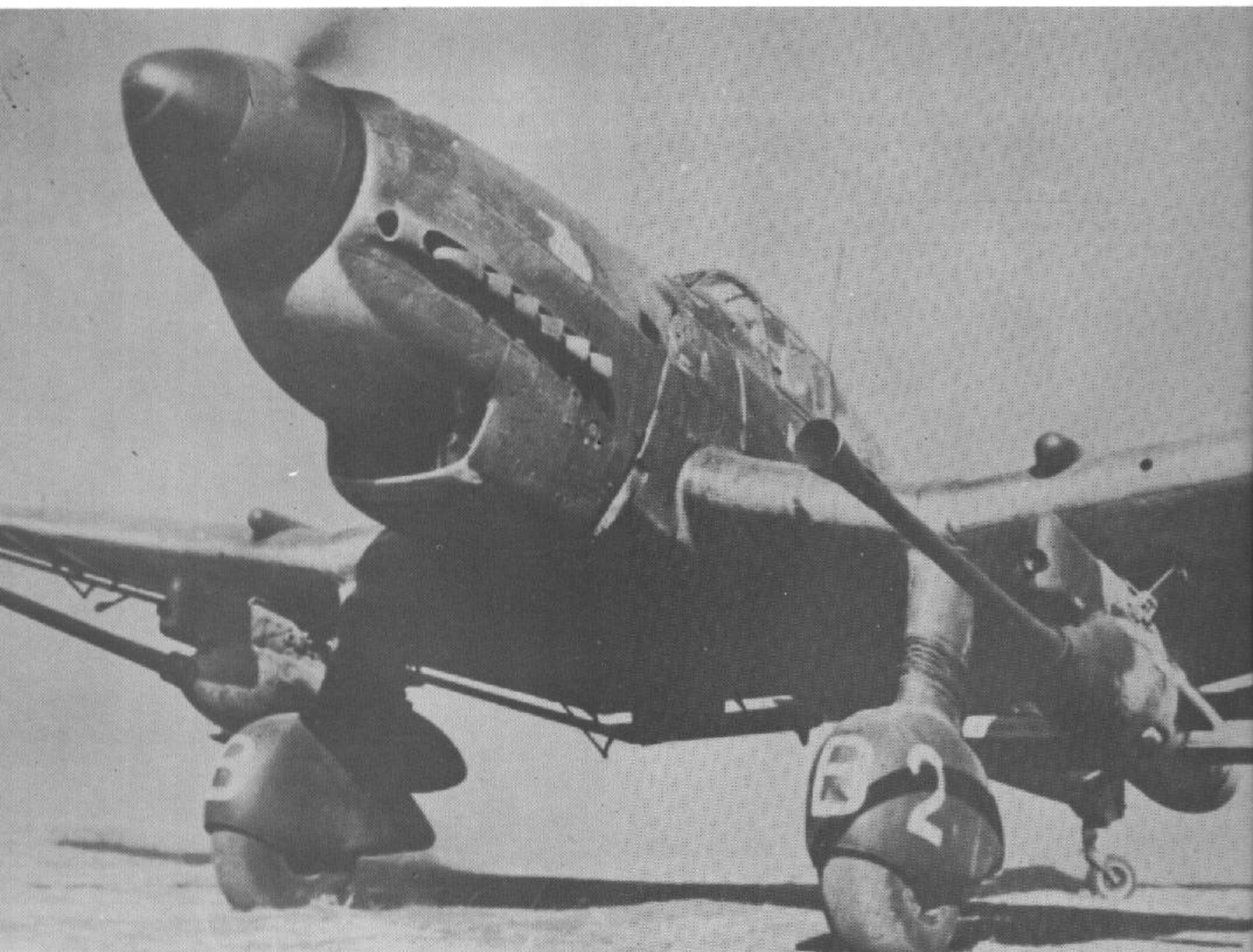
Ju 87 G-1 closeup. This model featured two 37 m m. Flak 18 cannon slung under each wing. This model had no dive flaps, and it was far from maneuverable, however, it was very successful against Russian Tanks.
