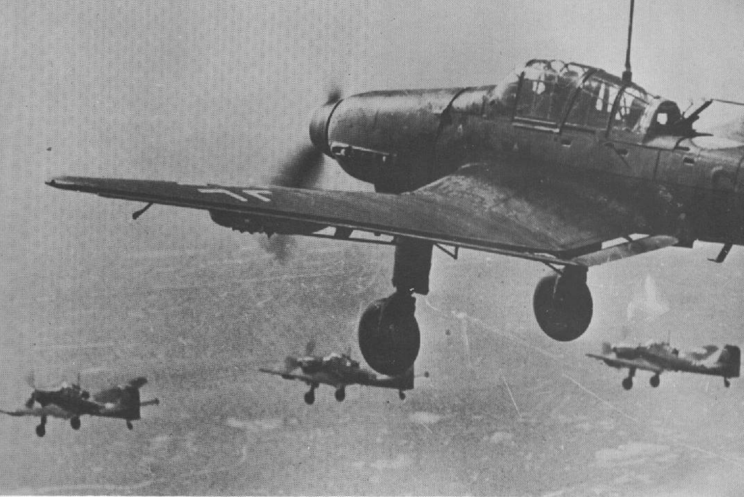
Flight of Ju 87 D-3's return from mission against Soviet strongpoints. The Ju 87 D series was extensively redesigned. It mounted the new powerful Jumo 211 engine of 1400 h.p.
