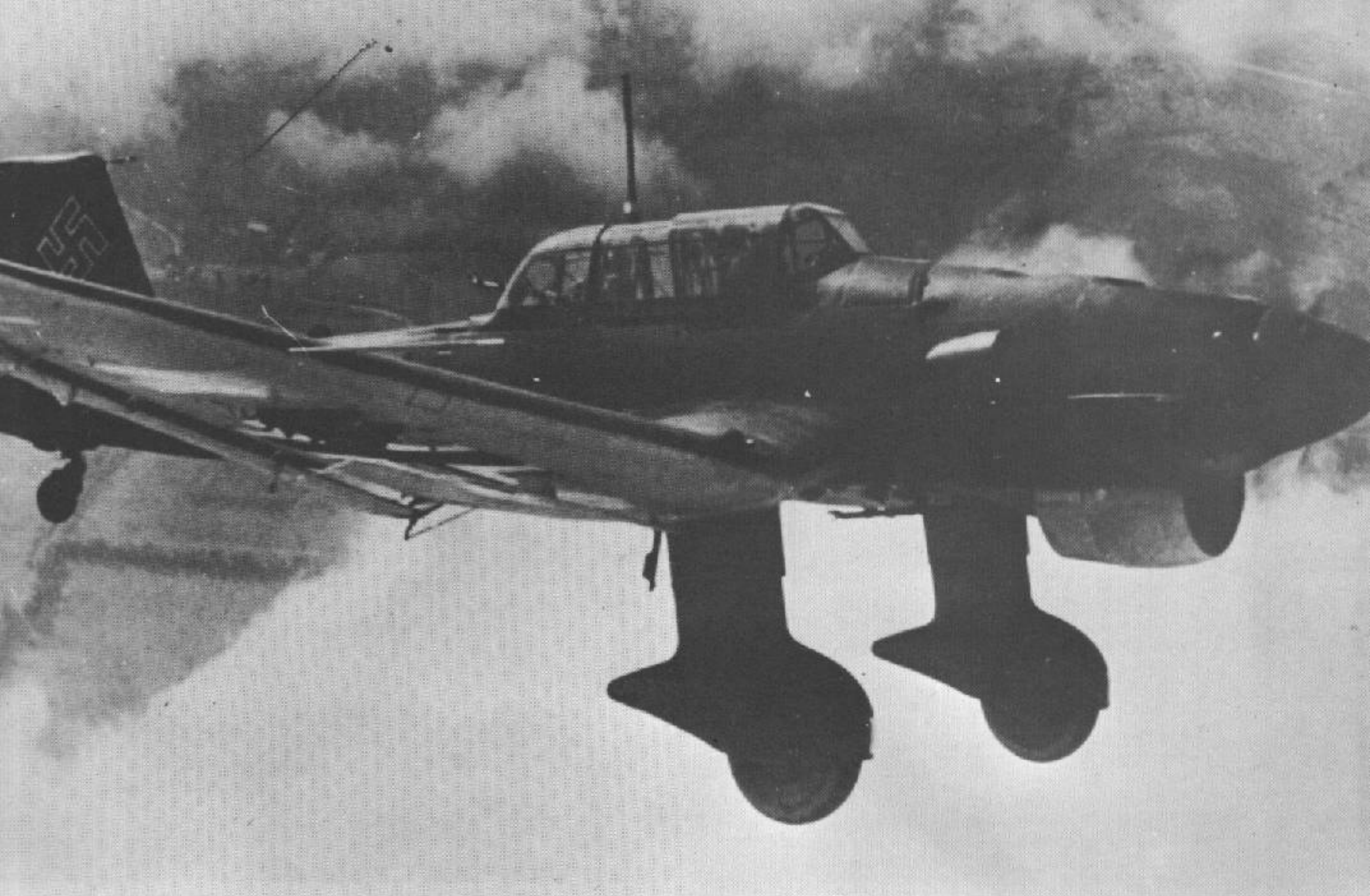
Ju 87 B-1 above gave way to the B-2 model which differed primarily in having larger propeller blades.
