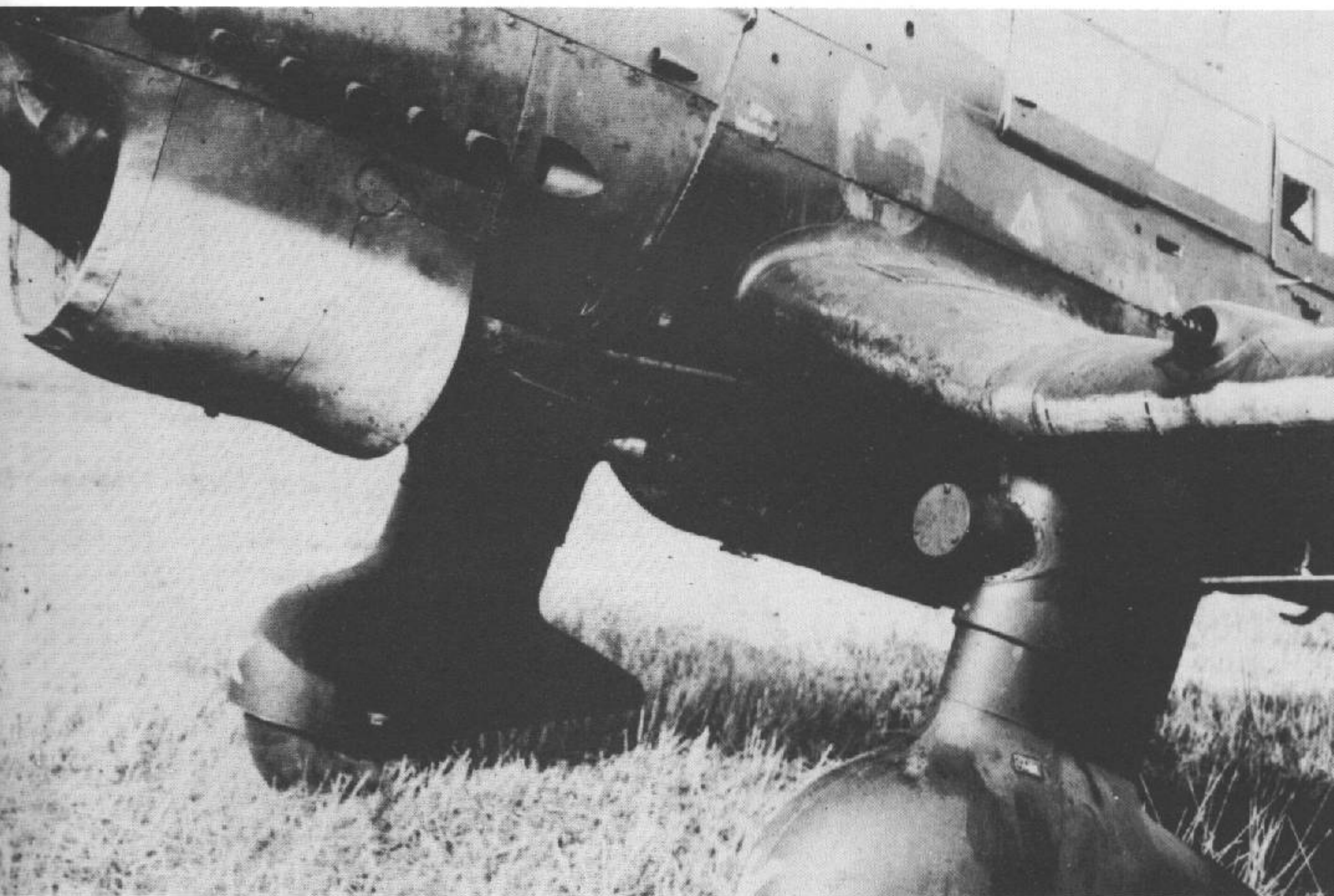
Ju 87 B-2 closeup showing bomb in position under belly and 7.9 m m. MG-17 wing machine gun. Siren on landing gear fairing has been removed and capped off.
