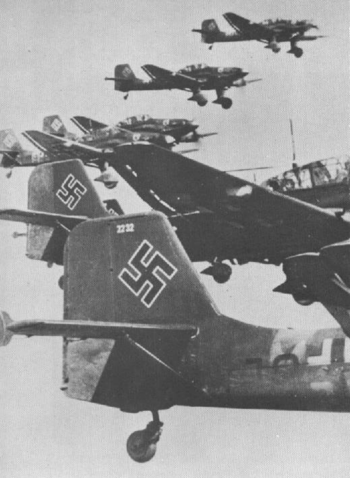
Lineup of Ju 87 D-1 Stuka's from the Immelmann Geschwader. The Ju 87D had a maximum speed of 255 m.p.h at 13,500 feet and a ceiling of 24,000 feet with a full bomb load.
