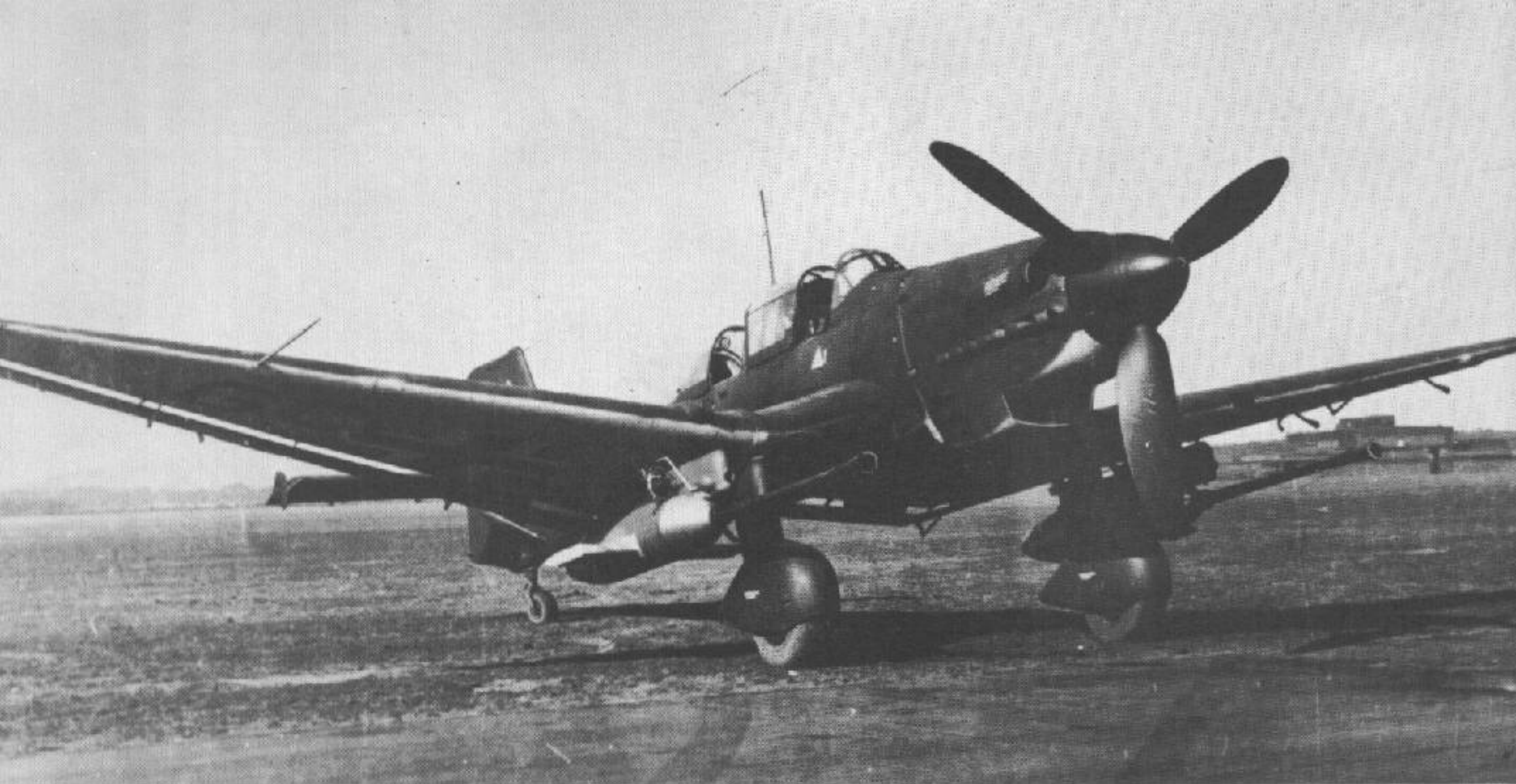
Last production model in the Stuka series the Ju 87 G-1 featured a new redesigned wing. Used principally as an anti-tank aircraft in Russia from 1942-1945, the Stuka proved to be a most effective tank killer.
