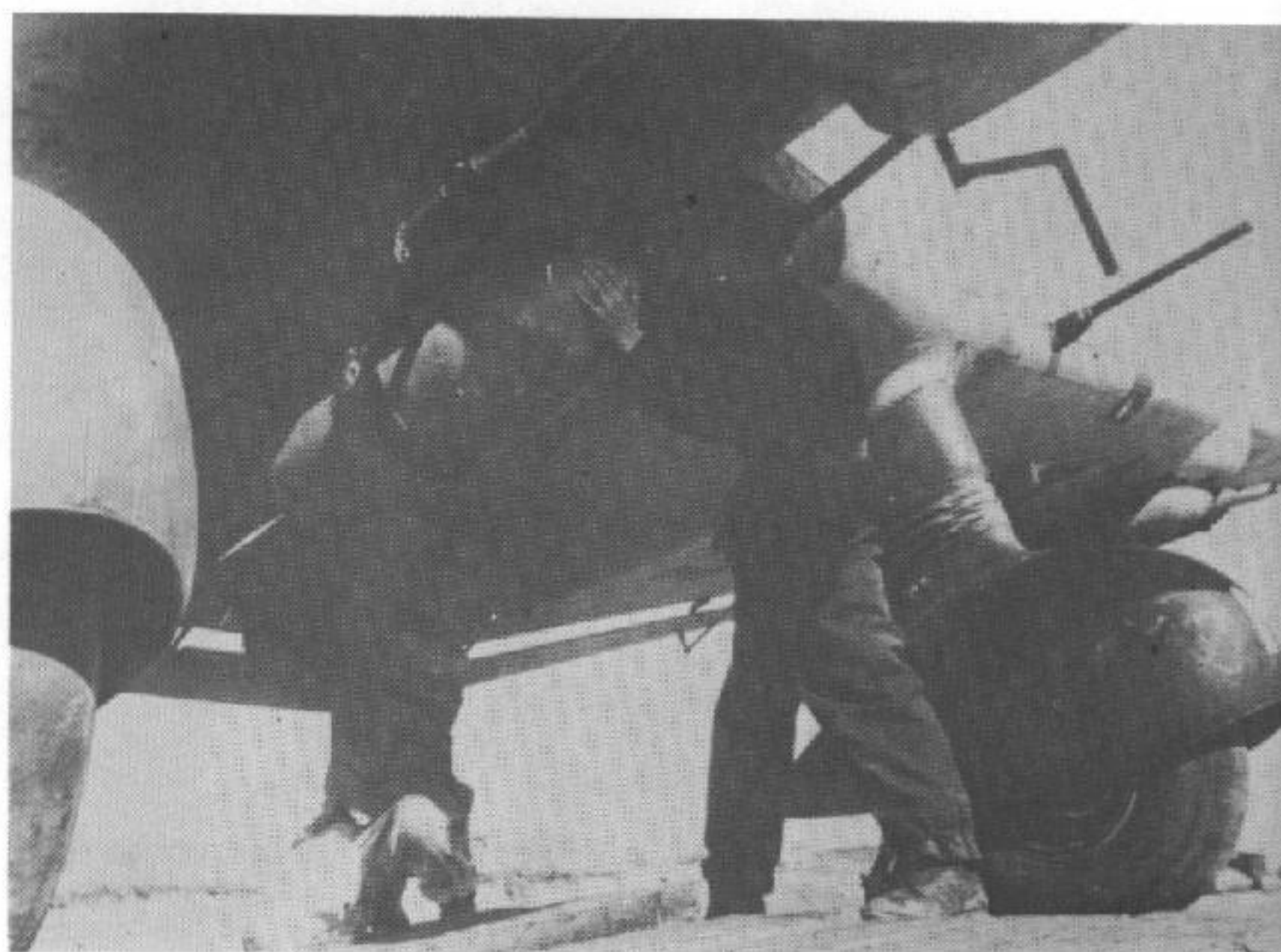
Two mechanics make final adjustments on 550 lb. bomb attachments in preparation for sortie against Russian target. Note starter crank extending down from Jumo engine.
