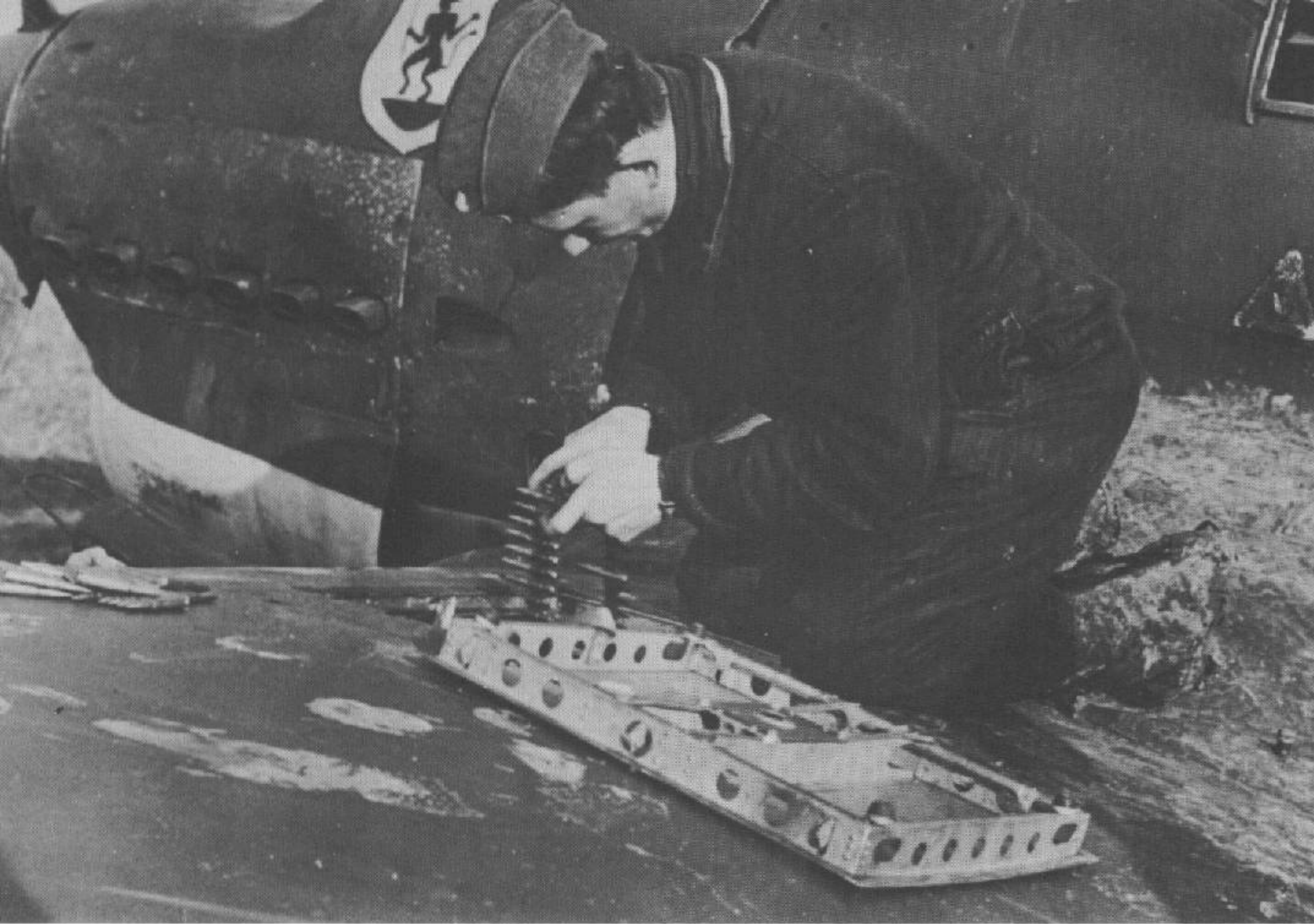
Stuka armor mechanic loads 7.9 m m. ammunition belt into the left wing MG-17 machine gun. Note 87 octane rating on fuselage side and Squadron insignia on front cowling.
