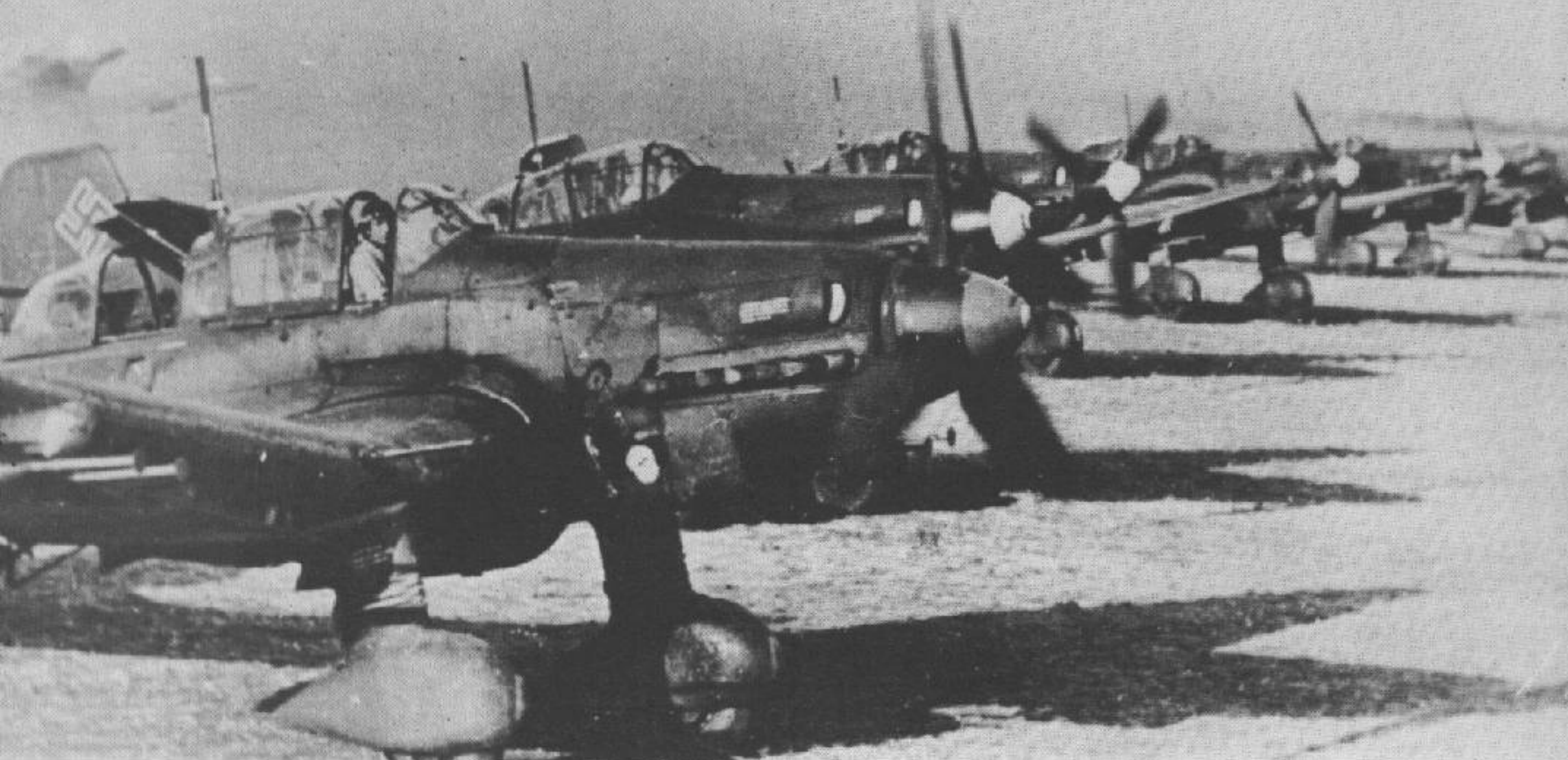
All bombed up and ready to go. These Junkers Ju 87 D-8 Stuka's are from Hans Ulrich Rudel's Stuka Unit. Note special long percussion detonators on the two outer 110 lb. wing bombs.
