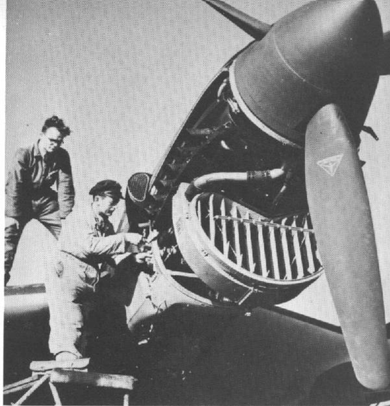
Junkers' mechanic adjusting Ju 87 B engine. Note coolant radiator engine air intake.
