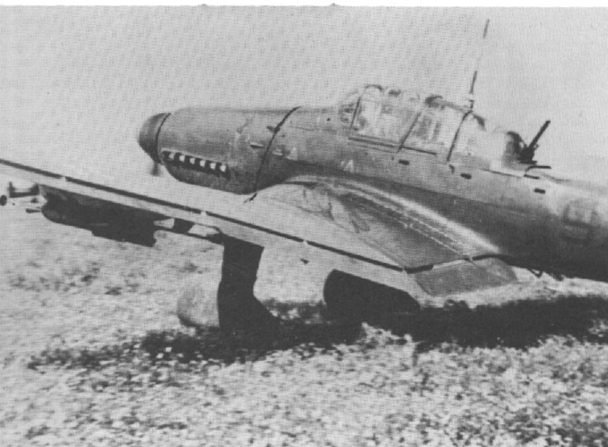
Ju 87 D-2 of 1./St. G.1 bombed up and ready for another sortie against Soviet troop concentrations, note special anti-personnel bombs under the wings.
