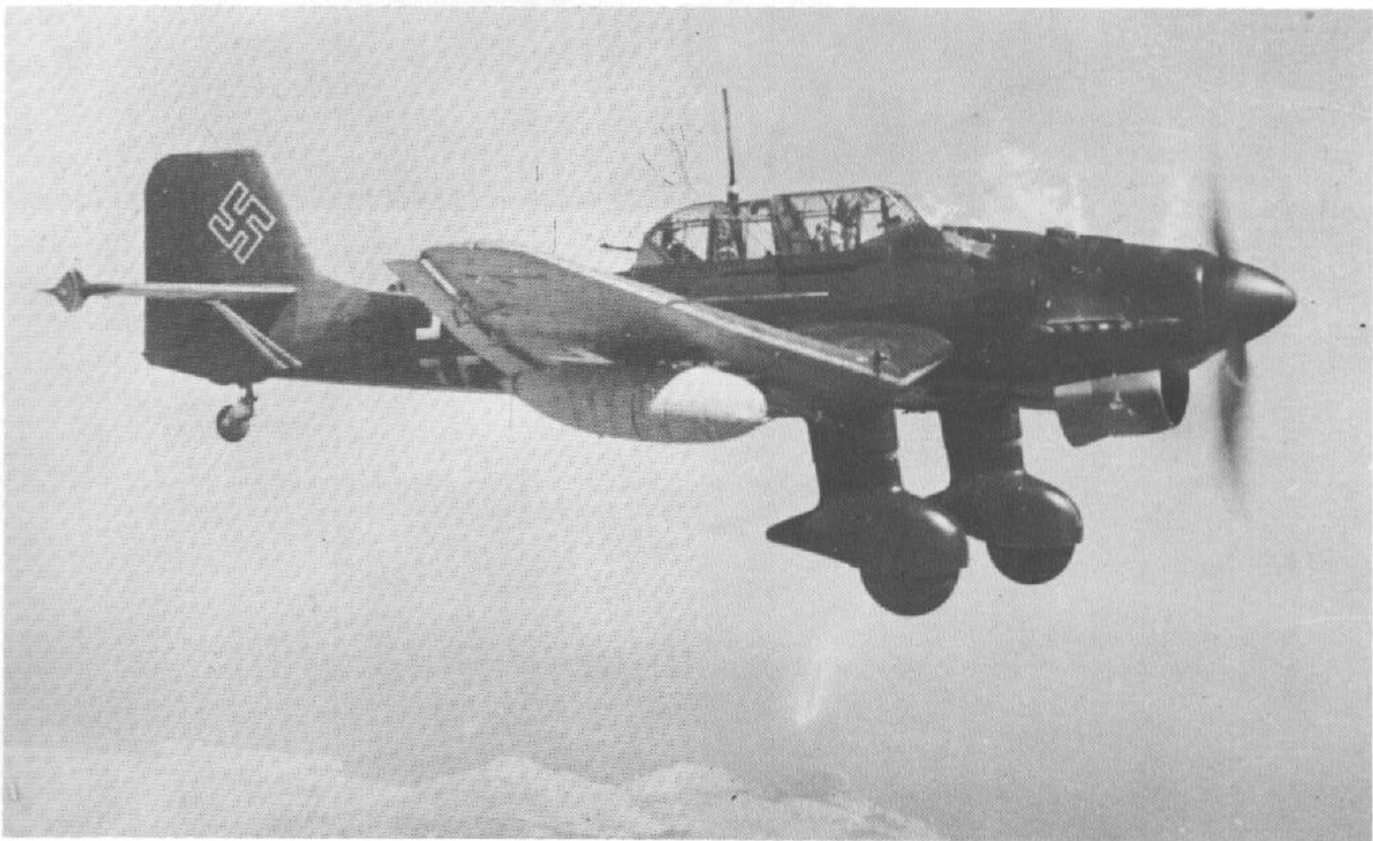
The Ju 87 R-2 had provisions for external fuel tanks. It had a range of 875 miles and was used extensively in attacks against the island fortress of Malta, from bases in Sicily.
