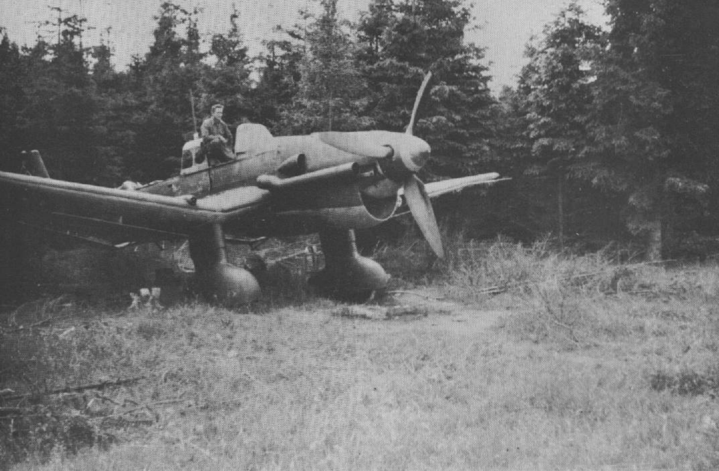
Junkers Ju 87 D-1 as captured in 1945 by American troops in a wood close to the Autobahn in Munich, Germany. Note special engine exhaust flame dampener installed for night missions.
