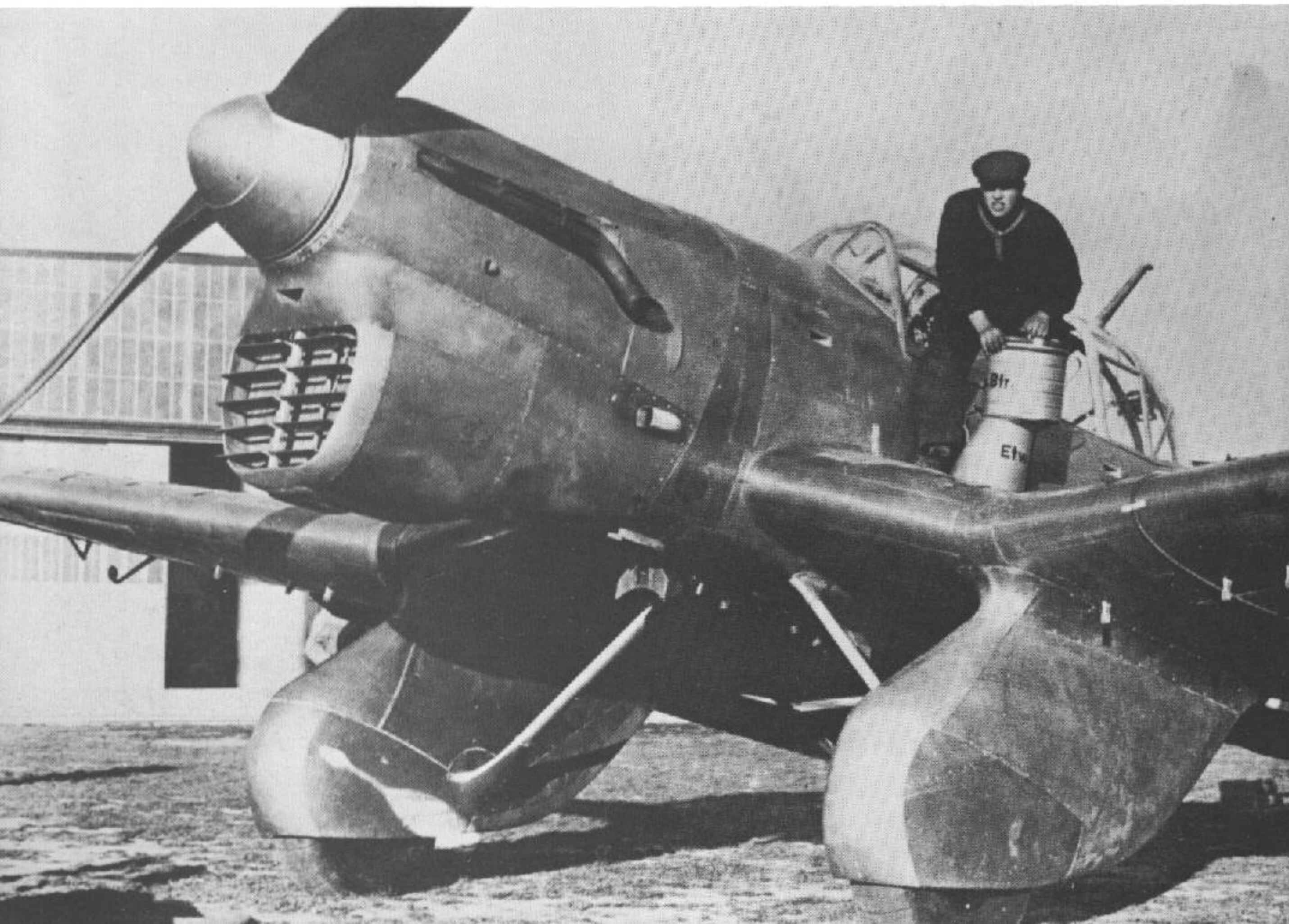
Design prototype of the Stuka series, the Ju 87 V-1 employed a British Rolls Royce Kestrel V engine.
