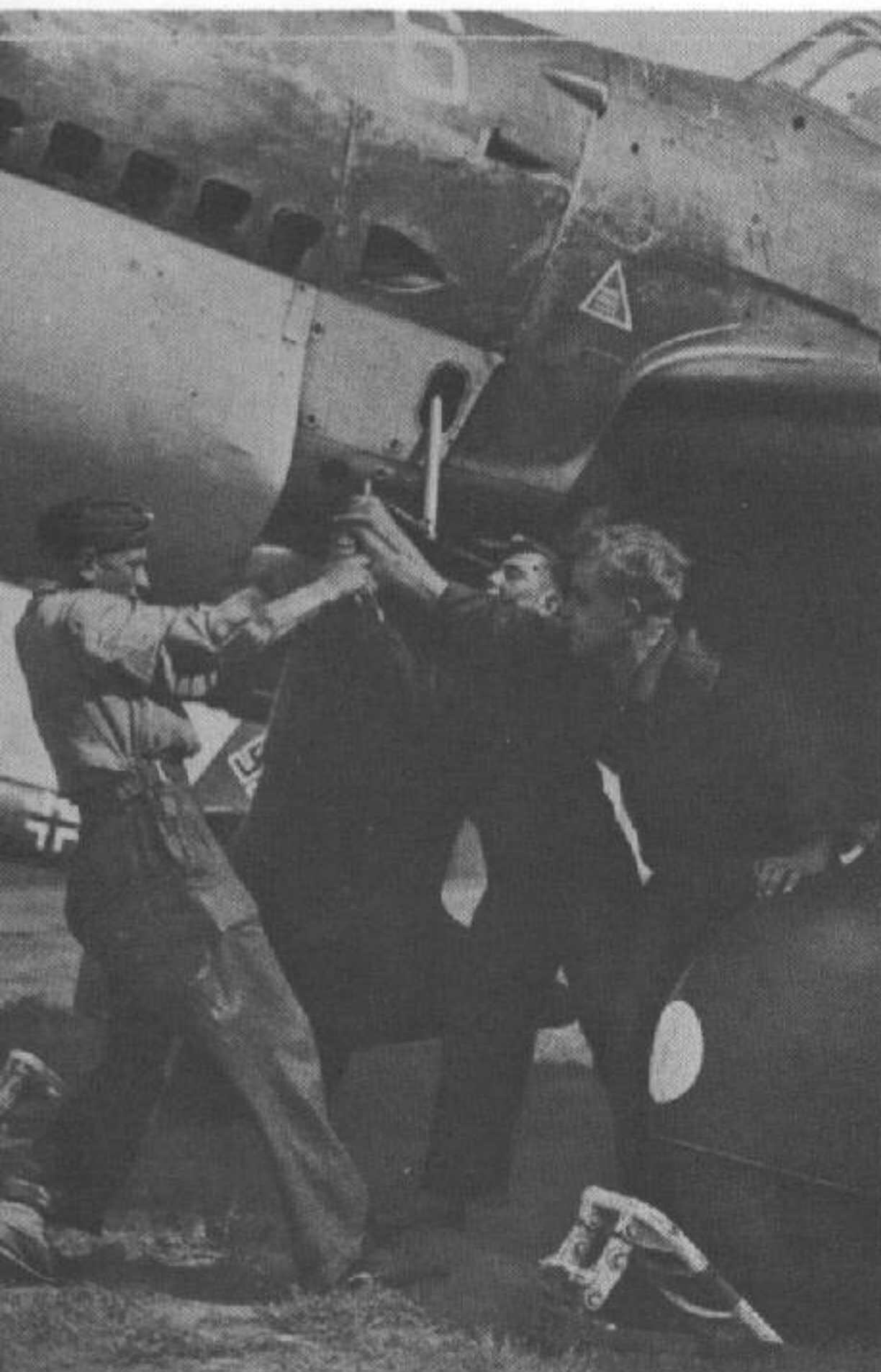
Luftwaffe mechanics pull through engine inertia starter crank in preparation to start Ju 87 B-2 Jumo engine.
